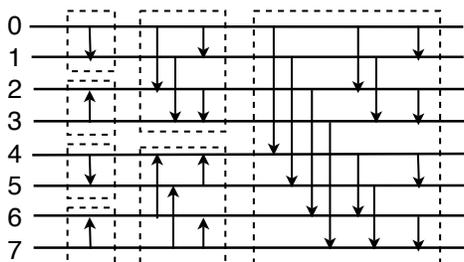
Figure 1: A bitonic sorting network of size  $N = 8$ . The network can be partitioned in three stages, each containing bitonic mergers of size 2, 4, and 8, respectively.
