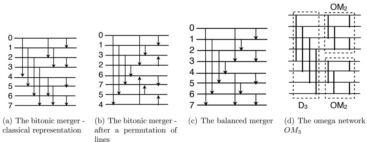
Figure 3: The bitonic merger, the balanced merger, and the omega network of size 8
