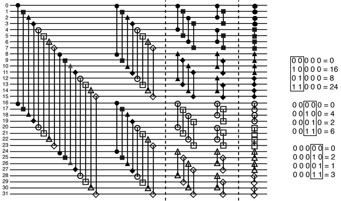
Figure 4: Three data layouts for the omega network  $OM_5$ .
